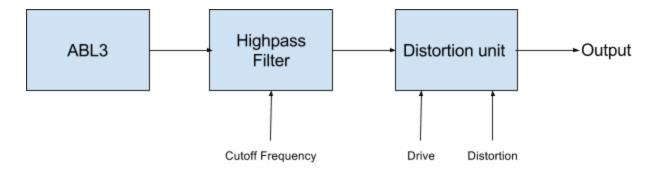
The distortion unit is an emulation of a transistor distortion circuit, which has the property of maintaining constant output power with different values of Drive.
